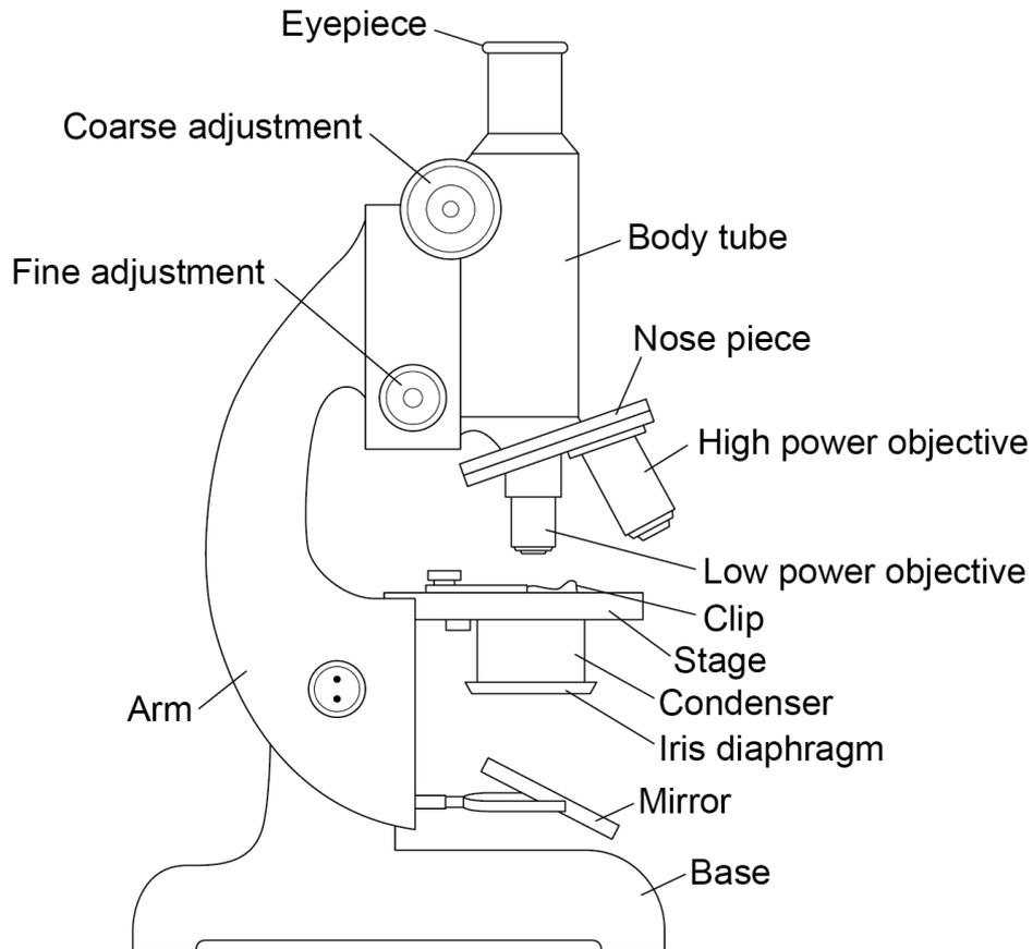
This microscope has a mirror to reflect light up through the slide. Some microscopes have a built-in light instead of a mirror.
