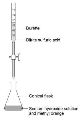
5. Carefully open the tap so that sulfuric acid flows into the flask at a drop by drop rate.
