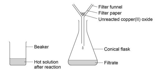
When filtration is complete, pour the contents of the conical flask into the evaporating basin.
