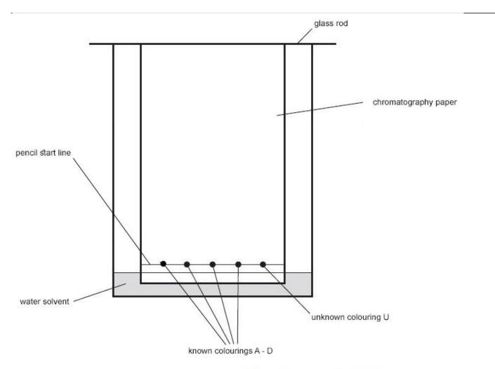
5. Wait for the water solvent to travel at least three quarters of the way up the paper. Do **not** disturb the beaker during this time.
