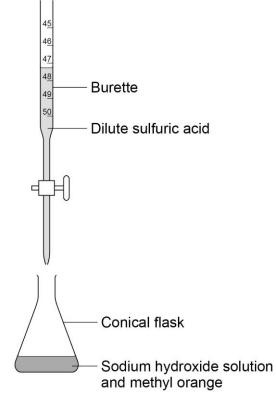
5. Carefully open the tap so that sulfuric acid flows into the flask at a drop by drop rate.
