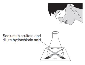
5. Write the time it takes for the cross to disappear in the first blank column of the table such as the one below. Record the time **in seconds**.
